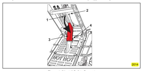
Figure 4-5 Install Safety Support
